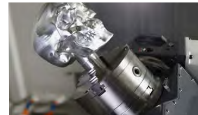
5th axis option is available on all XYZ Vertical Machining Centres except the LR Range.
