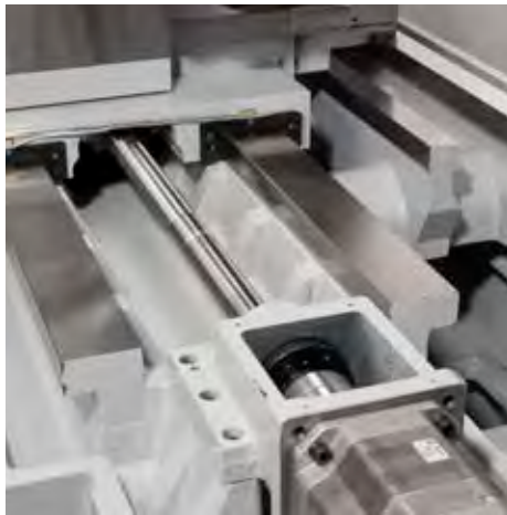
Box Slideways of the XYZ TC 320 LTY The 320 LTY is fitted with large hardened and ground guideways giving superb rigidity and performance.
