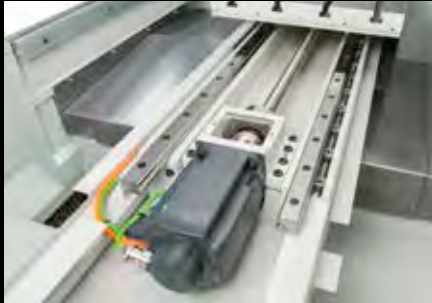
Linear Rails on all axes of the LR Range
